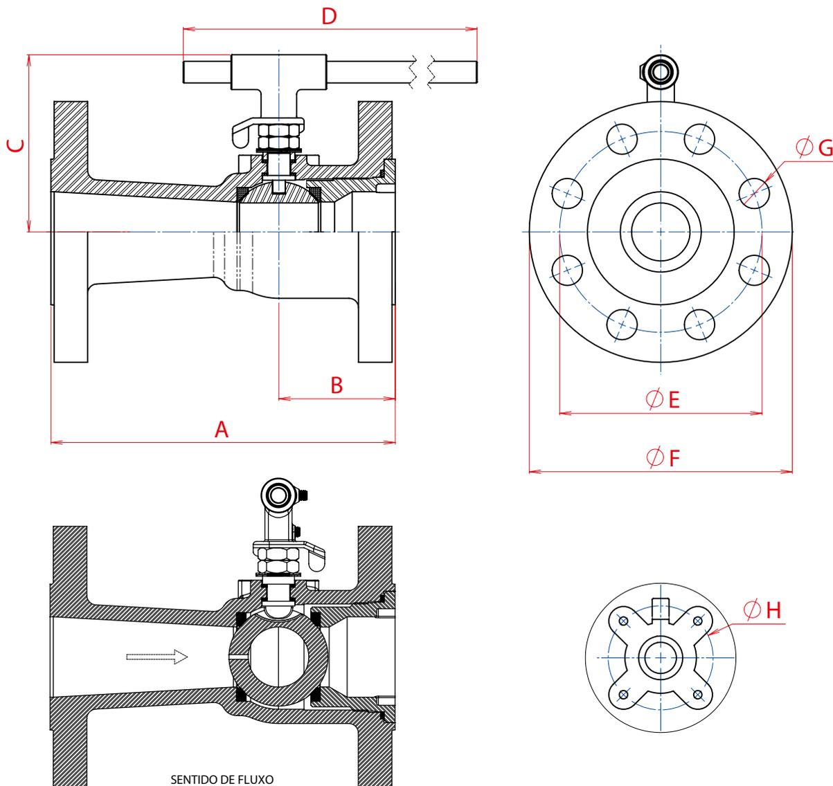
**VÁLVULA DE ESFERA MONOBLOCO PASSAGEM REDUZIDA (PR) CLASSE 150**
